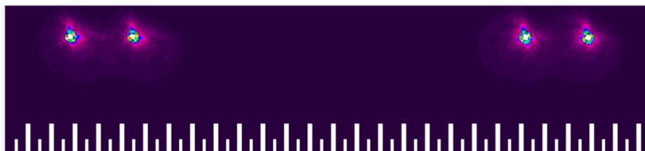
Fig. 4 FLDI beam pairs for a setup developed using diffractive optics and a 2-arcminute Wollaston prism. The major tick marks are at 100 \mu\text{m} , and the minor tick marks are at 50 \mu\text{m} .
